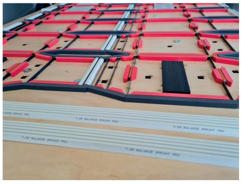
running an oversize sheet, and the die is kept in perfect condition without need for costly alterations. It also saves times for the operator and reduces tonnage and patch up. For die makers, Sprint Balance Pro replaces several production processes, requires less cutting rule, labour time and reduces laser time. Additionally, it eradicates the need for rubber on each side of the cutting rule and is highly cost effective.
