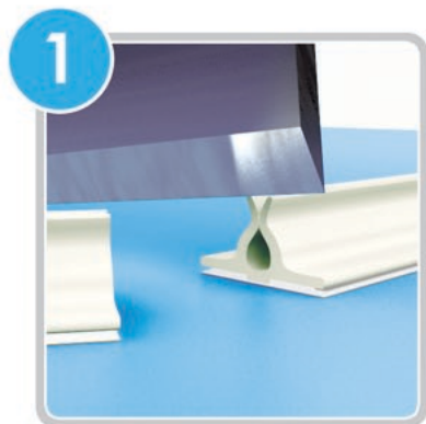
1 Cut Matrix to length of Creasing Rule
